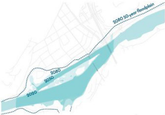
CLIMATE CHANGE IMPACTS: FLOODING, SEA LEVEL RISE (SLR) The design should ensure that Kingston waterfront is resilient to climate change impacts by designing for mitigation and adaptation. The 2020, 2050 and 2080 inundation and 50 year flood event is studied.
