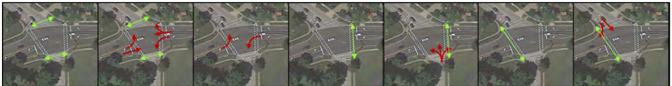
Figure 9: LPI and lagging left-turn phasing at Boston Mills Road / E Case Drive
