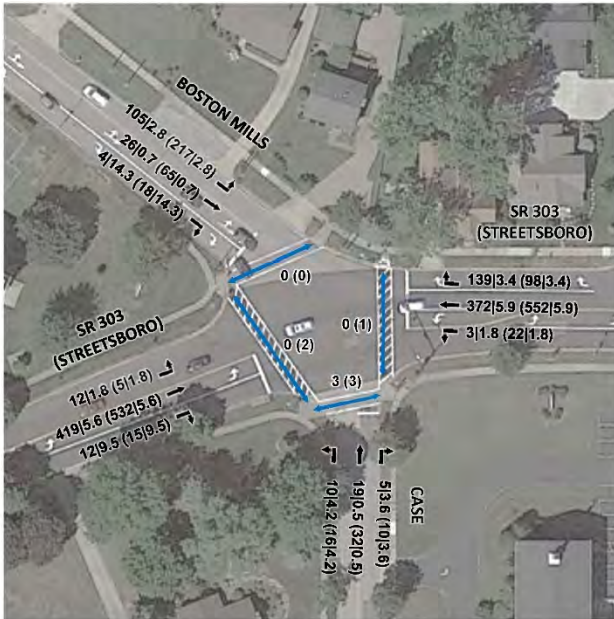
VEHICLE - AM VOLUME | HEAVY VEHICLE% (PM VOLUME | HEAVY VEHICLE%) PEDESTRIAN - AM VOLUME (PM VOLUME)
