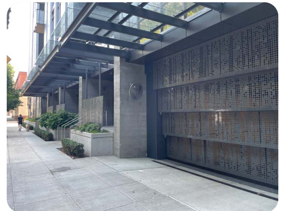
Parking entrances and loading docks should use the same materials as the main building to create a uniform architectural look. If possible, the building massing should ensure that they are slightly recessed from the main pedestrian path of travel.
