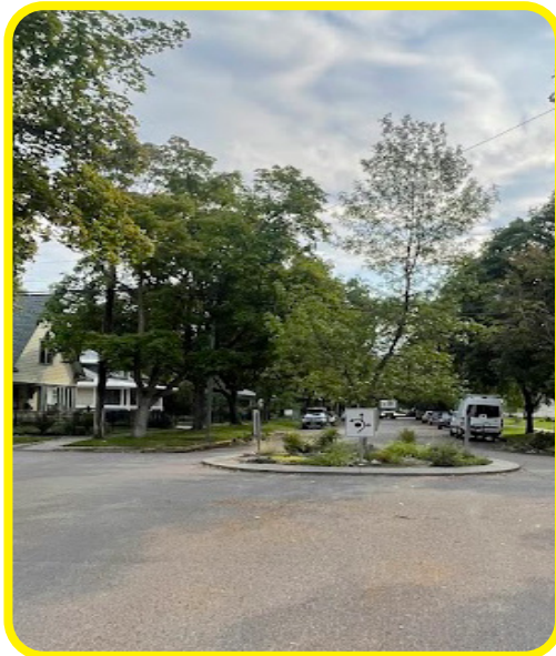
Traffic calming and management at intersections: permanent and quick-build traffic circles are one example. Others include bulb-outs. No center line markings, sidewalks on both street sides, tight curb radii, and unmarked crosswalks are also characteristic typical treatments of Neighborhood Residential streets.
