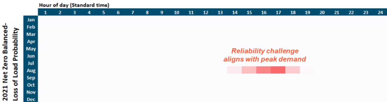
Figure 84. Loss-of-Load Probability Distribution by Month-Hour for the Net Zero Carbon Base Scenario in 2021
