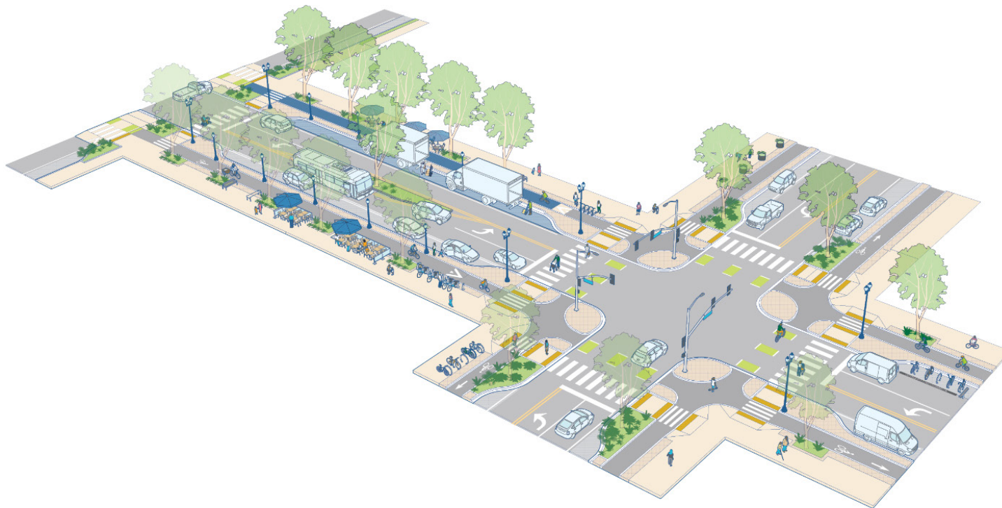
FIGURE 3-5 Roadway With Commercial Loading Zones
