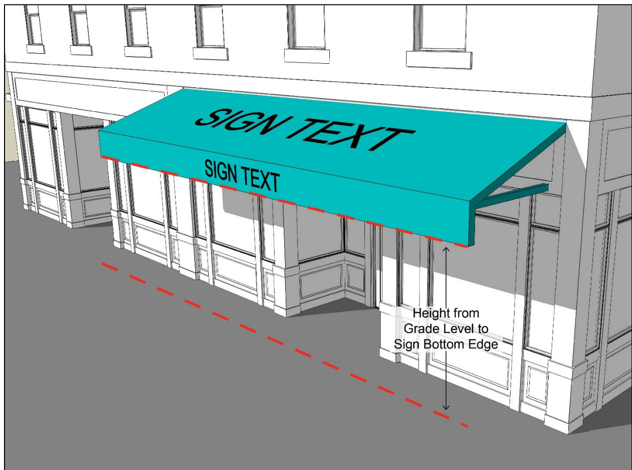
Figure 1104.04-D: Height to Sign Bottom Edge Measurement Example
