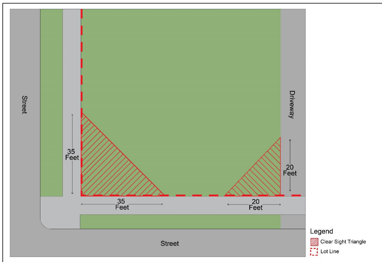
Figure 1115.05-A: Example Clear Sight Triangles
