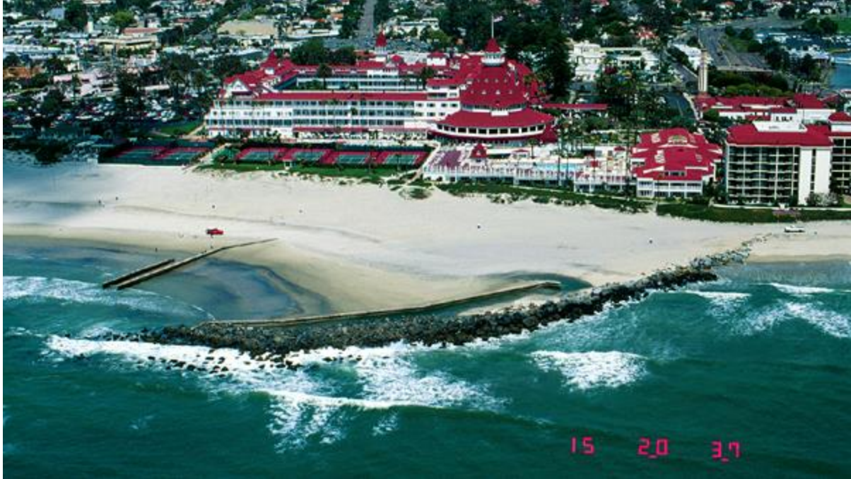
Figure VA-19: Erosion at the Hotel Del Coronado Groin – 1997/1998 El Niño Season (Patsch & Griggs, 2006)
